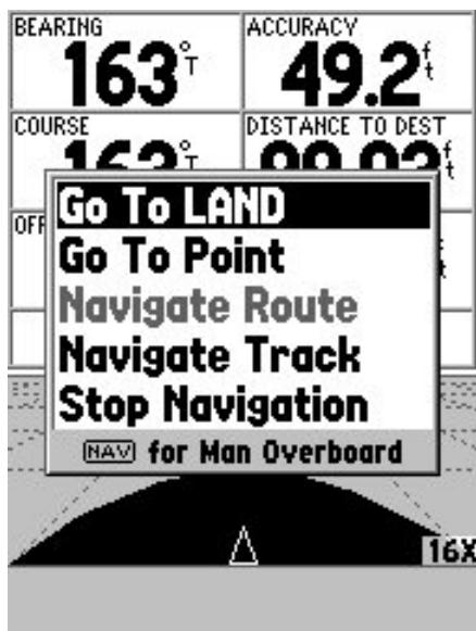
25. *Stop and verify the remaining distance and direction by pressing the <NAV> key which displays the Navigation Menu.”*
