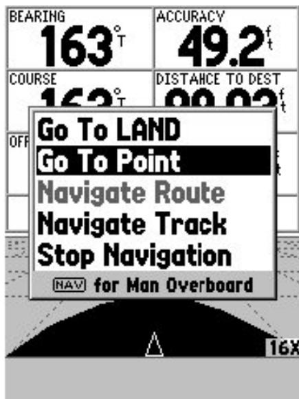
3. Using the <ROCKER> key, highlight “Go To Point” and press the <ENTER> key.
